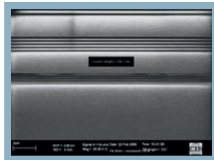
UV-NIL: 50nm, 70nm lines and spaces imprinted with MJB4 Mask Aligner. Courtesy: IHT, TU Braunschweig
