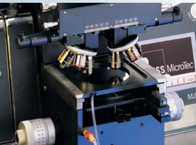
Optical System of a SUSS MJB4 Mask Aligner
