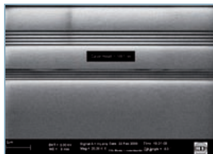
UV-NIL: 50nm, 70nm, 100nm lines and spaces imprinted with MJB4. Courtesy: IHT, TU Braunschweig
