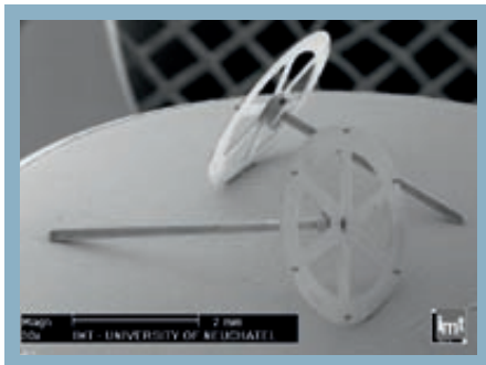
Piezo motor for MEMS applications Courtesy: IMT, University of Neuchatel
