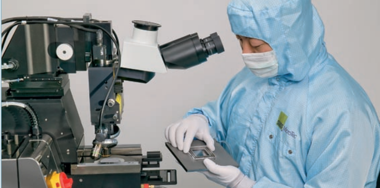
The UV-NIL toolkit for SUSS Mask Aligners enables patterning of sub-50nm geometries
