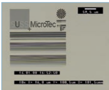
SUSS MicroTec logo printed in Amonil MMS4 on a SUSS Mask Aligner
