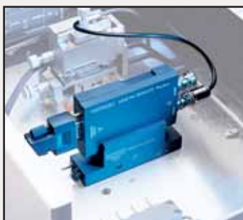
PreAmps can be mounted on the probe station with either a platen base or a triax mounting bracket. By reducing the signal path between the DUT and the PreAmp from several feet to a fraction of an inch, the Model 4200-SCS can eliminate cable effects like parasitic capacitance and leakage currents, for more accurate low-level measurements.
